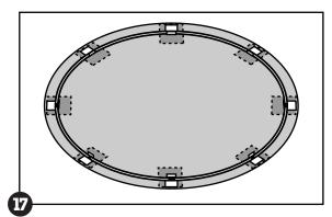
c. Remove the base rails and base plates and lay out the patio stones around the circle where the base plates were.
