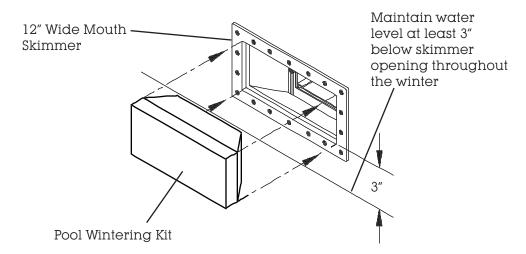
Insert the Pool Winterizing Kit (Part Number 1370138) into the skimmer until it fits flush with the skimmer flange. On some skimmers, it may be necessary to trim the foam to make a friction fit and/or use a wooden wedge to keep it in place during the winter.
