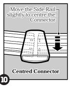
connector and loosen the screws on the side rail. Shift the side rail in or out from the centre of the pool until the connector can be properly centred between the rails (see diagram 10).
