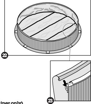
5. Fasten the Liner in place (V-Bead Liner only)
