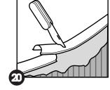
Roll up any excess liner hanging below the plastic coping and tape it in place near the top of the pool wall. Important: Do not trim off the excess liner.
