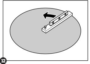
d. Remove all the high spots with a shovel, hoe or rake. Be prepared to hire earth moving equipment if you need to level a large area. Remember, your pool must be level within 1" (25 mm) across the diameter of the pool.
