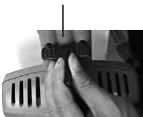
Pushing in retaining clips with plastic tool (provided)
