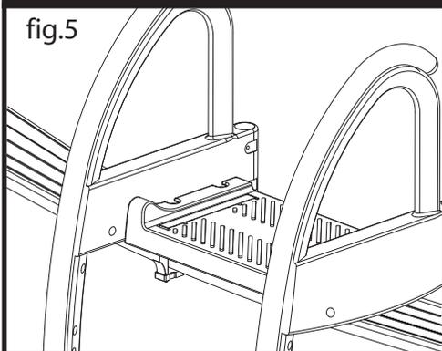
5- Lower the assembled portion of the ladder until it rests on the top rail. Fix the platform to the top rail of the pool introducing the straps into the opening of the platform and under the top rail. (fig.5)
