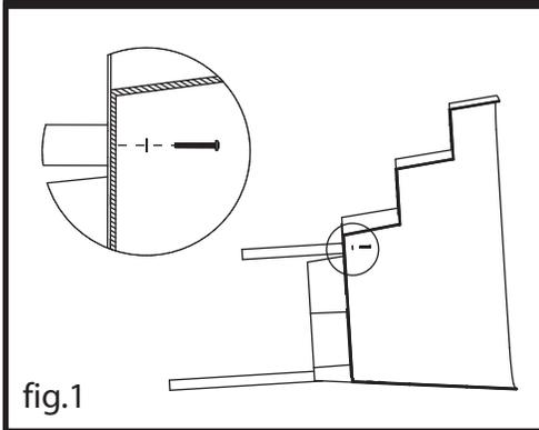
1- Put the step on the side to fix the short support rail on the step. Screw from the inside using the predilled hole with the 2 1/2 bolt(1), and washer(1). (fig.1)
